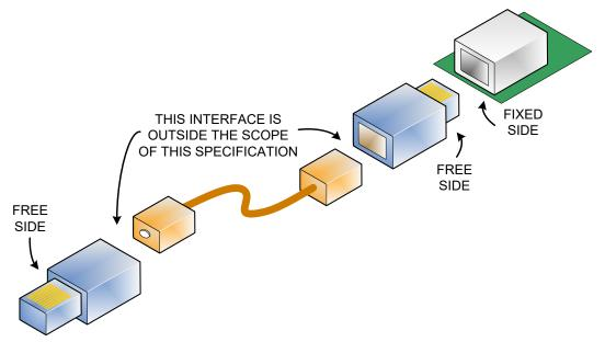
Figure 4-3 Separable Transceiver Module Implementation
