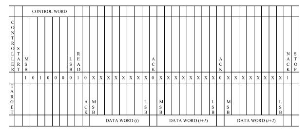
Figure 5-5 Sequential Address Read Starting at Current Address
