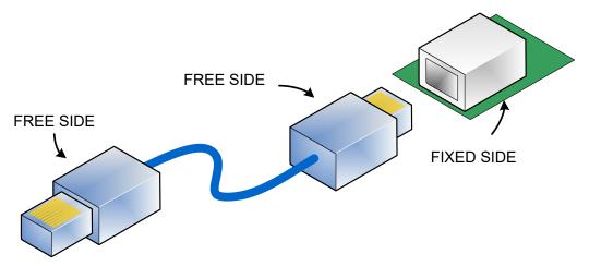
Figure 4-2 Cable Assembly Implementation
