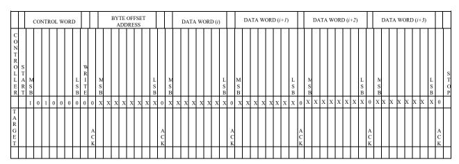
Figure 5-2 Sequential Write Operation
