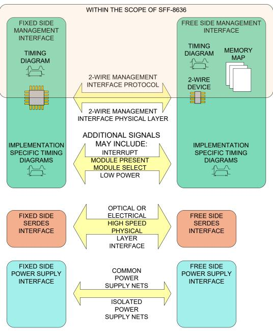
Figure 4-1 Common Management Interface Block Diagram
