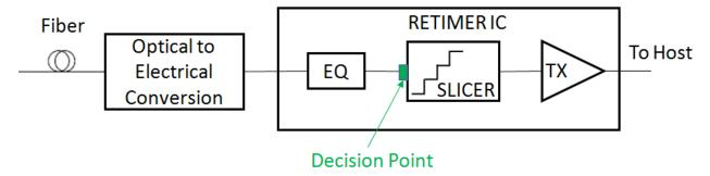
Figure 6-1 Optical ingress path of Module
