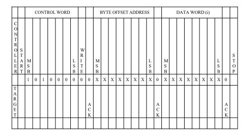
Figure 5-1 Write Byte Operation
